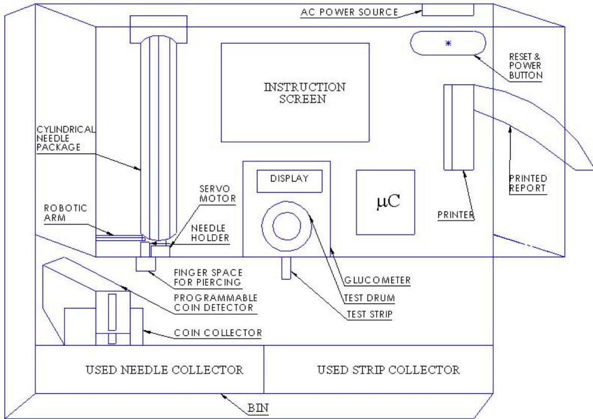
Fig. 10 Coin based automated blood sugar level monitoring system
