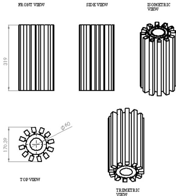
Fig. 15 construction and dimensions of the needle package
