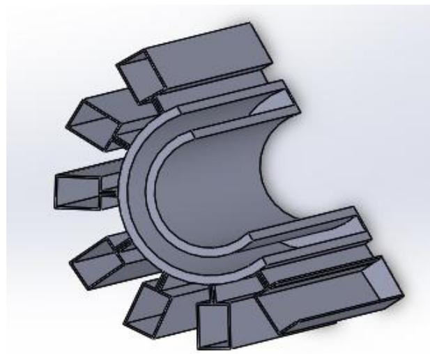
Fig 16 Cut section view of the cylindrical needle package
